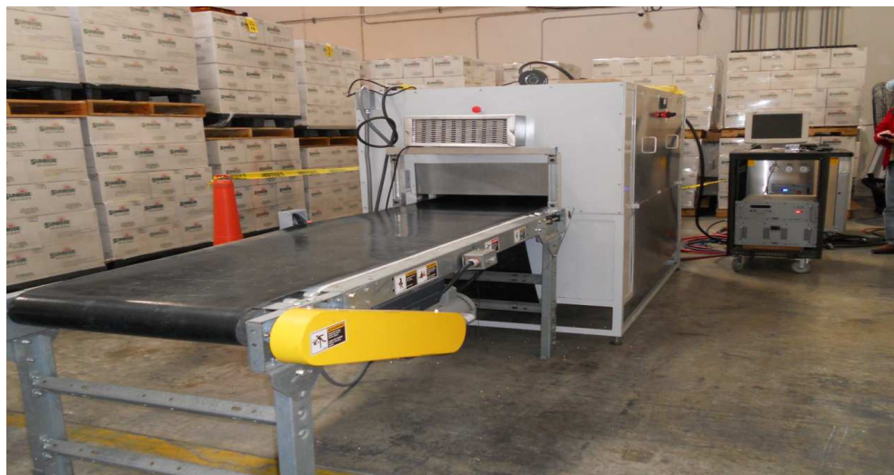
Fig. 4. RF system for batch processing (13.15 MHz, 10 kW). Designed by UC Davis & RF Biocidics Inc.
