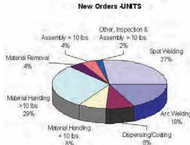
Fig. 1. 2003 Robot Applications in North America . A total of 12,367 robots valued at $876.5 million were ordered. When sales to companies outside North America are added in, the total for North American robotics suppliers is 12,881 robots valued at $913 million. NOTE: These numbers include results from North America and Outside North America. Source: Robotic Industries Association.
