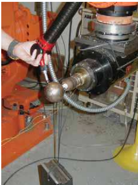
Fig. 15. Experiment Setup for robot stiffness measurement.
