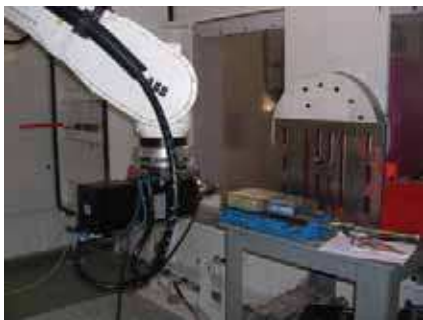
Fig. 12. Setup for robotic deburring.
