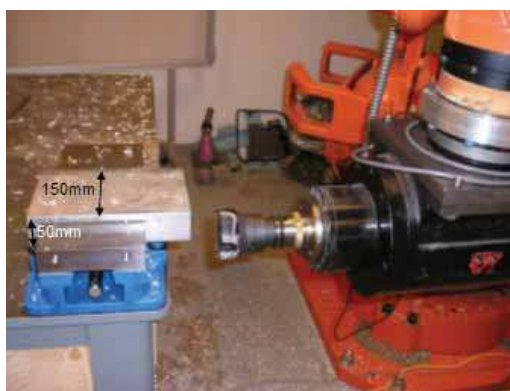
Fig. 18. Experimental setup for robotic milling.
