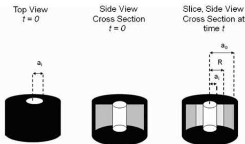
Fig. 2. Diagram of a hollow cylindrical matrix device:  $a_i$  was the inner radius;  $a_o$  was the outer radius;  $R$  is the distance to the interface between the drug depletion zone (light gray area) and the drug dispersing zone (dark gray area); and black representing coated regions through which the drug release could not take place (Reproduced from Wiranidchaphong, 2006).
