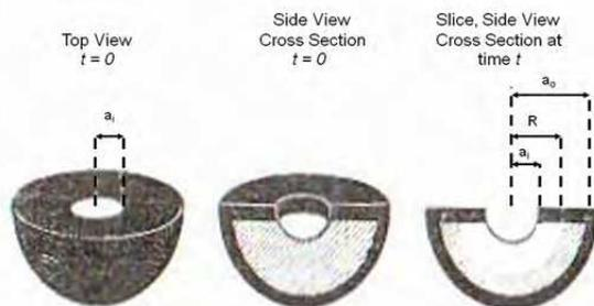
Fig. 1. Diagram of a hemispheric polymer matrix device:  $a_i$  was the inner radius;  $a_o$  was the outer radius;  $R$  was the distance to the interface between the drug depletion zone (white area) and the drug dispersing zone (diagonal lines); and black represented coated regions through which the drug release could not occur (From Hsieh, et. al., 1983).
