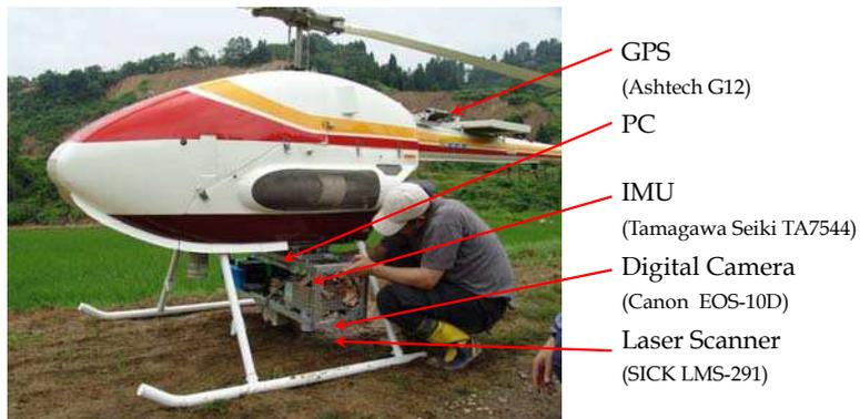
Fig. 10. UAV, model RPH2 made by Fuji Heavy Industries, Ltd.
