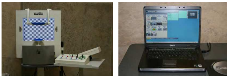
Fig. 4. Electrophysiology unit: Monitor, showing checker-board for stimulation, amplifier and laptop with several softwares for different tests.
