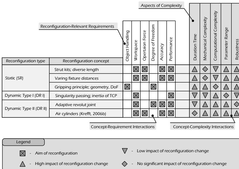
Fig. 18. Reconfiguration-approach-matrix.
