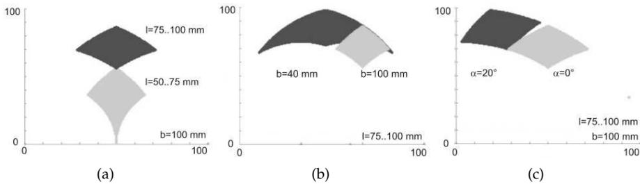
Fig. 8. Influence of the reconfiguration parameter on the position and dimension of the workspace: a) varied strut length  $l_1, l_2$ ; b) varied frame diameter  $b$  and c) varied angle  $\alpha$  at the frame connection level.
