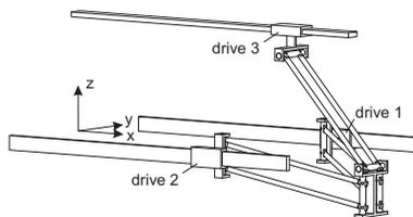
Fig. 9. Kinematic structure of the TRIGLIDE robot.
