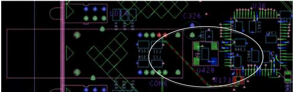
Fig. 16. Unrouted differential lines.
