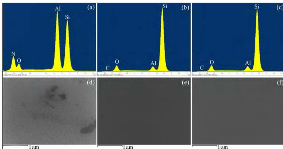
Fig. 6. EDX spectra and FESEM images of AlN thin films grown from metal target (a, d), ceramic target in Ar atmosphere (b, e) and ceramic target in a mixture of Ar and N<sub>2</sub> (c, f).
