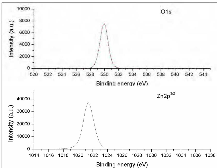
Fig. 2. O1s and Zn2p<sup>3/2</sup> XPS peaks acquired after surface cleaning on ZnO\_MR sample. The dotted red line represents the peak fitting the O1s peak.
