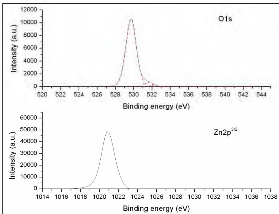
Fig. 3. O1s and Zn2p<sup>3/2</sup> XPS peaks acquired after surface cleaning on ZnO\_CN sample. The dotted red lines represent the peaks fitting the O1s peak.
