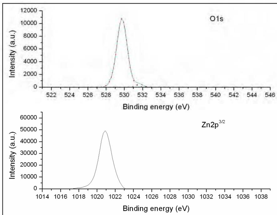
Fig. 4. O1s and Zn2p<sup>3/2</sup> XPS peaks acquired after surface cleaning on ZnO\_CR sample. The dotted red lines represent the peaks fitting the O1s peak.
