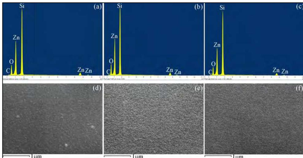
Fig. 1. EDX spectra and FESEM images of ZnO thin films grown from metal target (a, d), ceramic target in Ar atmosphere (b, e) and ceramic target in a mixture of Ar and O<sub>2</sub> (c, f).
