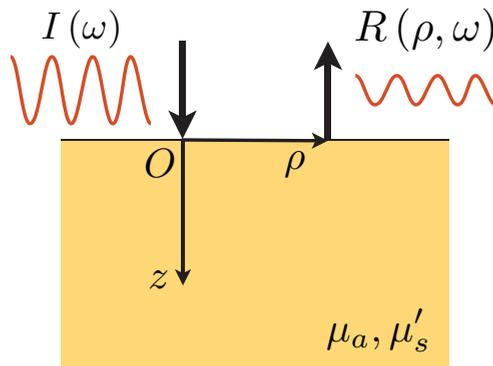
Fig. 4. Scheme of reflection geometry FD-NIRS measurement. Intensity modulated light  $I(\omega)$  travels in the medium and part of it can be collected by a detector at a source-detector distance  $\rho$ . Amplitude and phase of the collected light  $R(\rho, \omega)$  depend on  $\mu_a$  and  $\mu'_s$ .
