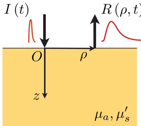
Fig. 5. Scheme of reflection geometry TD-NIRS measurement. Injected light travels in the medium and part of it can be collected by a detector at a source-detector distance  $\rho$ . Knowing the temporal shape of the injected light  $I(t)$ , the temporal shape of the collected light  $R(\rho, t)$  depends on  $\mu_a$  and  $\mu'_s$ .
