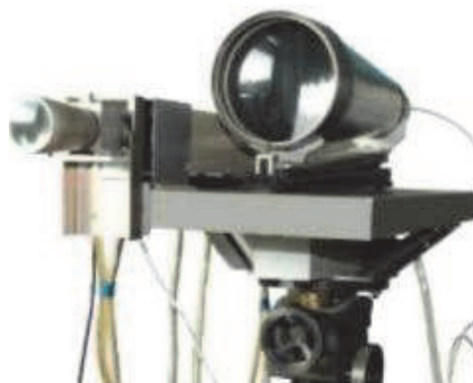
Fig. 1. The lidar scheme, with a separated transmitter and receiver.
