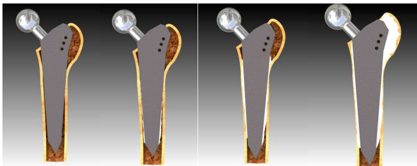
Fig. 2. Showing the process of gradual stem loosening as a result of hypertrophy of interface membrane (white) leading eventually to stem subsidence ( reproduced by courtesy of Jiri Lostak, MD )
