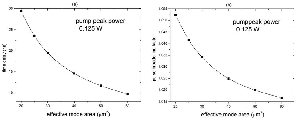
Fig. 10. (a) Time delay and (b) pulse broadening as a function of effective mode area at a given pump power.
