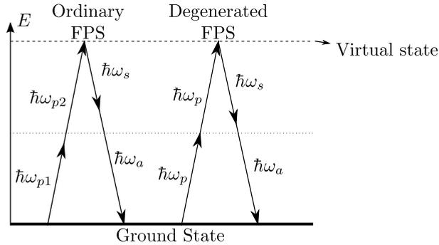
Fig. 3. Spontaneous four-photon scattering processes in silica fibers: ordinary and degenerated case.
