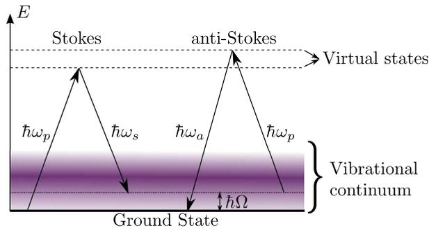
Fig. 1. Spontaneous Stokes and anti-Stokes processes in amorphous silica fibers
