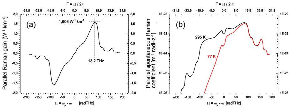
Fig. 2. (a) Raman gain  $g_{\parallel}$  in a silica fiber for  $\lambda_p = 1.5 \mu\text{m}$  and forward propagation. Peak value:  $g_R = 1.6 \text{ W}^{-1} \text{ km}^{-1}$ . Peak position:  $\Omega_R = 13.2 \text{ THz}$ . (b) Spontaneous Raman coefficient  $R_{\parallel}$  for  $\lambda_p = 1.5 \mu\text{m}$  and forward propagation at  $T = 295 \text{ K}$  and  $77 \text{ K}$ .
