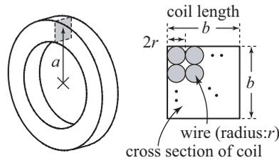
Fig. 7. Coil configuration.
