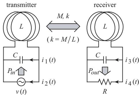
Fig. 3. Power transmission by magnetic resonant system.
