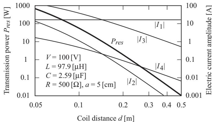
Fig. 5. Transmission power  $P_{res}$  and current amplitudes.
