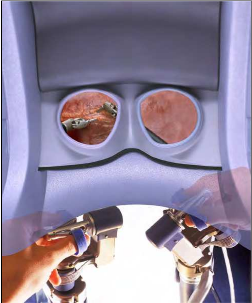
Fig. 4. The view through binoculars, a three-dimensional image
