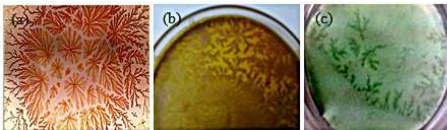
Fig. 6. Fractal aggregates of different sizes in (a) chitosan (b) PEO and (c) PVDF-HFP based electrolyte membranes
