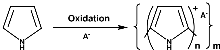
Fig. 1. Simplified mechanism of the polymerization of polypyrrole.
