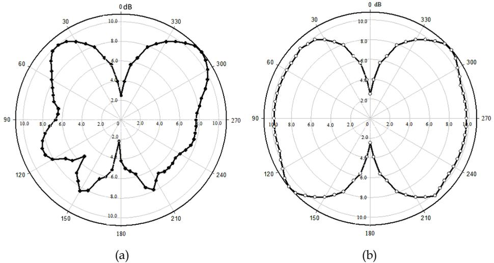
Fig. 6. Broadside divisive radiation patterns (a) Measured (b) Simulation
