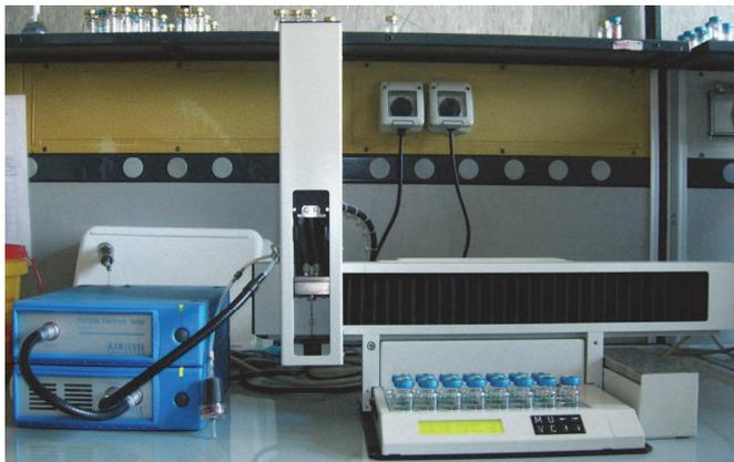
Fig. 1. An example of electronic nose.
