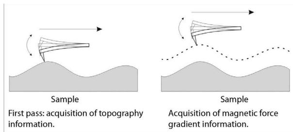
Fig. 4. Principle of operation of atomic force microscope.
