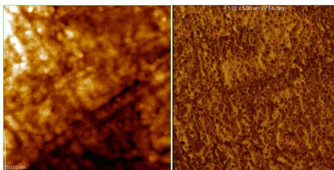
Fig. 8. Magnetic Force Microscopy: scan size is  $5 \times 5 \mu\text{m}$ . Left: topography image with maximum profile height of 150.9 nm. Right: the magnetic force gradient image of the same area. This image shows changes in magnetic force gradient, exhibiting that magnetic behaviour exist on the para- and diamagnetic levels and that they are inhomogenous in our samples (that are chemically homogenous).
