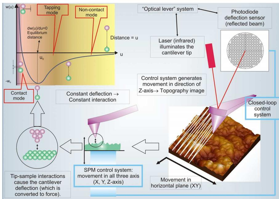
Fig. 3. Principle of operation of atomic force microscope.
