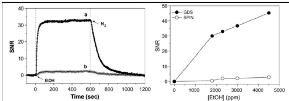
Fig. 16. (left) Single exposure/recovery cycle for GDS (a) and SPIN (b) films of Fe(TPP)Cl exposed to 2300 ppm EtOH ( $T = 20^{\circ}\text{C}$ ). (right) Calibration curves of SPIN and GDS films of Fe(TPP)Cl upon exposures to EtOH atmospheres over the range 1800–4500 ppm.
