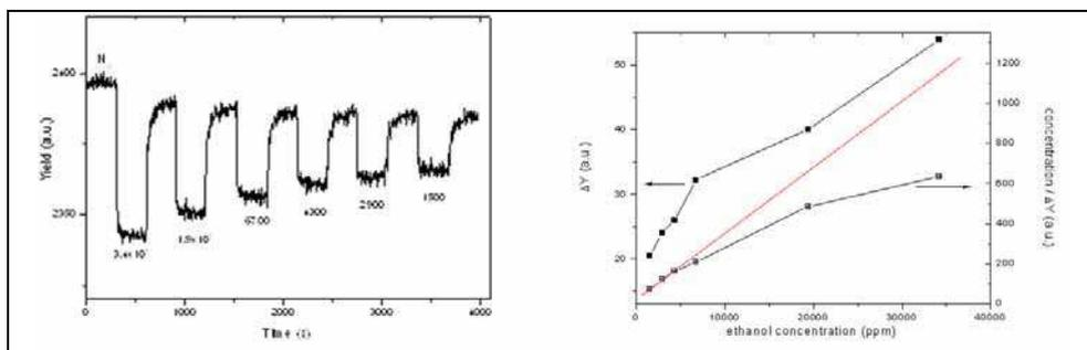
Fig. 4. (left) Optical response of CuPc sample towards different ethanol vapour concentrations at  $\lambda=580$  nm. (right) Calibration curve and Langmuir plot of CuPc sample towards ethanol at  $\lambda=580$  nm.
