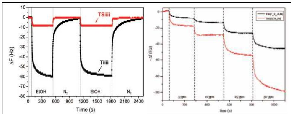
Fig. 19. (left) Change of the resonance frequency of VE Tiiii and TSiiii samples as a function of time during exposure to 25 ppm EtOH ( $T = 20^\circ\text{C}$ ). (right) Change of the resonance frequency of SPIN Tiiii[ $\text{C}_{11}\text{H}_{23}$ , H, Ph] and VE Tiiii [H,  $\text{CH}_3$ , Ph] samples at increasing amount of EtOH.
