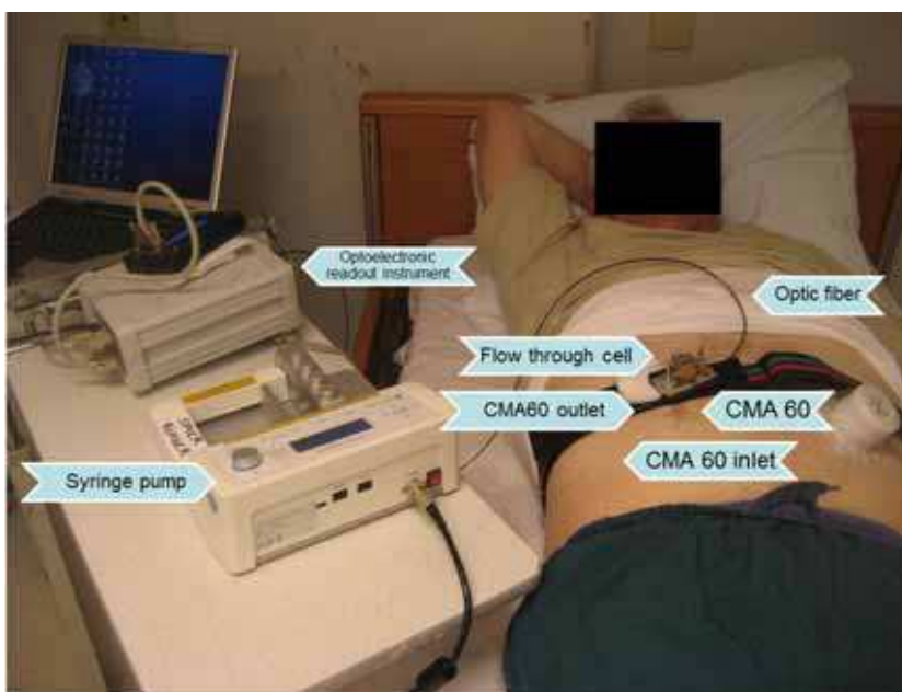
Fig. 4. Use of the optochemical oxygen sensor instrumentation during a typical in vivo experiment. The main components are the flow-through-cell, which is fixed near the umbilicus of the volunteer close to the position of insertion of the CMA 60 microdialysis catheter. The luminescence emitted by the oxygen sensitive membrane is collected by an optic fibre cable and guided to the optoelectronic read-out unit. The microdialysis probe is perfused using a microinfusion syringe pump. These experiments were carried out in the laboratory of Dr. G.H. Goossens (Maastricht University Medical Centre, The Netherlands).
