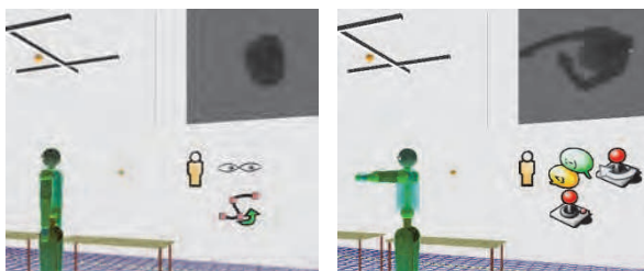
Fig. 9. Left: Human agent is watching the robot. Recognized situation: Monitoring. The robot is expected to carry on with its task of following a planned path. Right: Human agent is communicating. The complex action to signal a left turning movement is recognized. The robot is expected to comply with user instructions.
