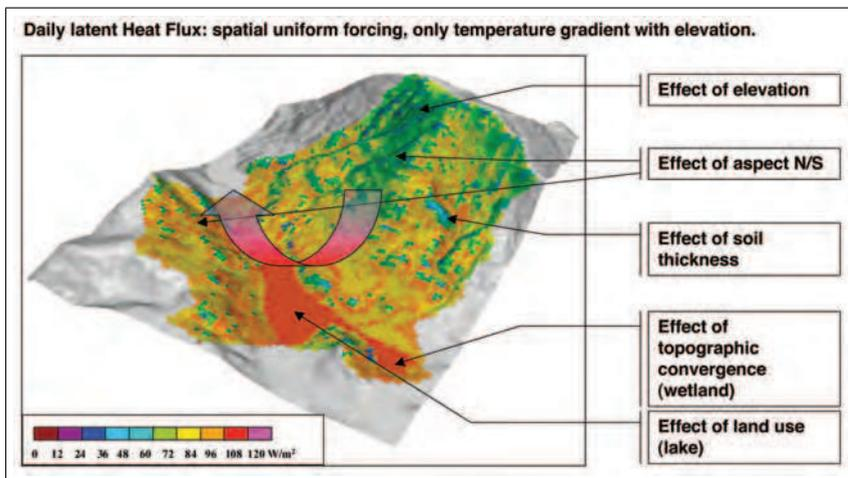
Fig. 8. Example of evapotranspiration  $ET$  for the Serraia basin, Italy. Notice the elevation effect (areas more elevated have less evaporation); the aspect effect (more evaporation in southern slopes, left part of the image); the topographic convergence effect on water availability (at the bottom of the valley).
