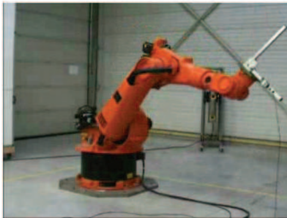
Fig. 9. Minimum of 3 LEDs are attached the tool frame during the calibration to obtain complete pose (6D). (Courtesy of Metris).
