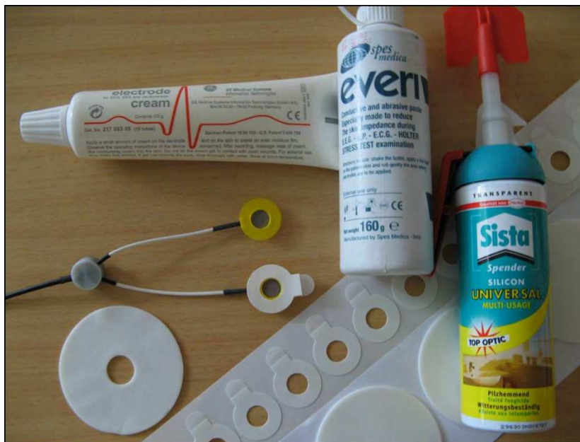
Fig. 2. WaS- EMG electrodes intended for water environments with accessories (Pánek et al., 2010).
