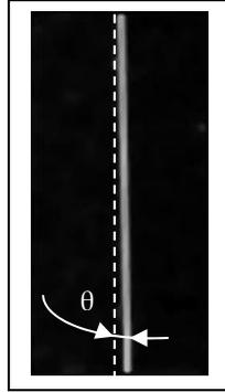
Fig. 3. Result of Sobel edge detection operator followed by thresholding and binary morphological processing (filtering) to identify the proper edge orientation ( $\theta_p \sim 0.95^\circ$ , for  $\theta = 1^\circ$ ).
