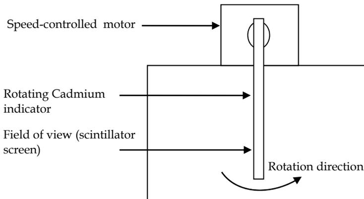
Fig. 9. Experimental arrangement for induced motion blurs characterisation.
