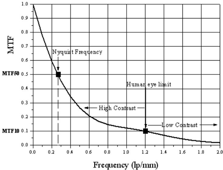
Fig. 7. MTF of the studied neutron imaging system.
