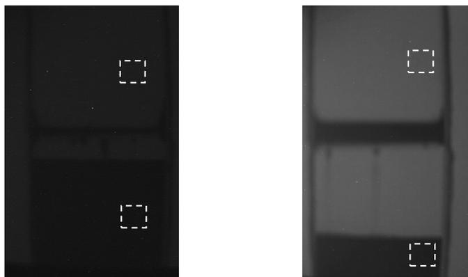
Fig. 16. Frames taken respectively from video sequence 1 and 2 of the water flow process for a frame rate of 12.5 fps, a Gain of 22 dB and a respectively neutron beam intensity of  $1.6 \times 10^6$  n/cm<sup>2</sup>/s and  $1.44 \times 10^7$  n/cm<sup>2</sup>/s (from the left).
