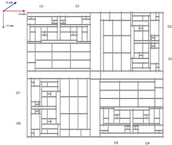
Fig. 9. The extracted IBM POWER4 MCM floor plan
