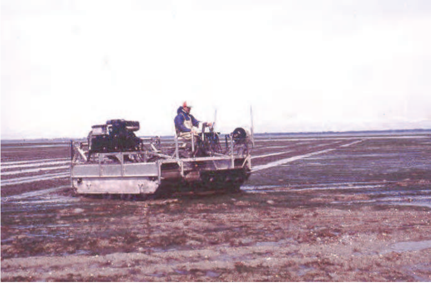
Fig. 5. Seeder machine combined to remove oyster shells
