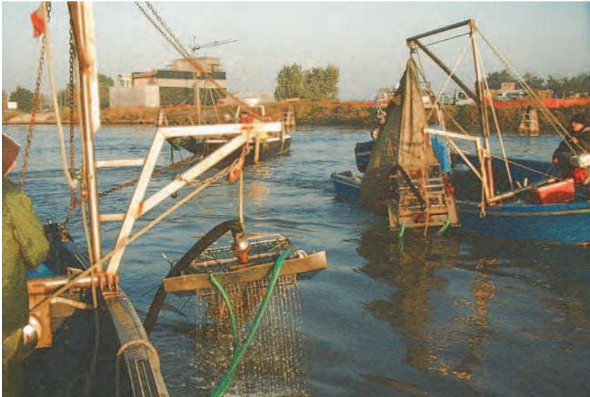
Fig. 9. Hydraulic clam dredge “idrorasca”
