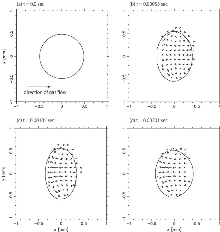
Fig. 8. Time evolution of molten droplet exposed to the gas flow. The gas flow comes from the left side of panels. We use  $p_{fm} = 10^4 \text{ dyn cm}^{-2}$ ,  $r_0 = 500 \text{ nm}$ , and  $\mu_d = 1.3 \text{ poise}$  for calculations.
