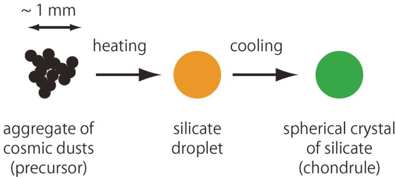
Fig. 1. Schematic of formation process of a chondrule. The precursor of chondrule is an aggregate of  $\mu\text{m}$ -sized cosmic dusts. The precursor is heated and melted by some mechanism, becomes a sphere by the surface tension, then cools to solidify in a short period of time.
