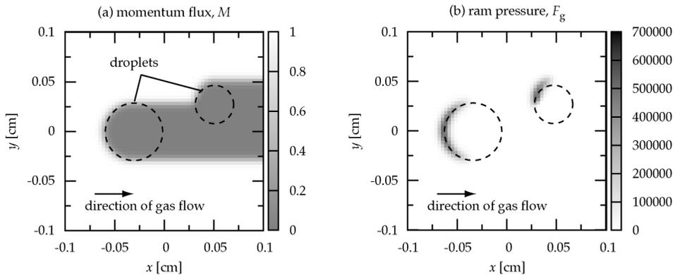
Fig. 7. Spatial distributions of the momentum flux  $M$  (a) and the ram pressure  $F_g$  (b) of the free molecular gas flow around a spherical droplet in  $xy$ -plane. The dashed circles are sections of the droplet surfaces in  $xy$ -plane. Units of the gray scales are  $p_{fm}$  for the panel (a) and  $\text{dyn cm}^{-3}$  for the panel (b), respectively. We adopt  $p_{fm} = 5000 \text{ dyn cm}^{-2}$  in this figure.
