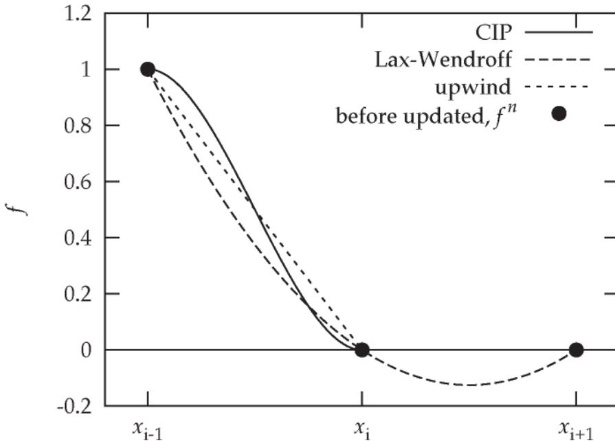
Fig. 5. Interpolate functions with various methods: CIP (solid), Lax-Wendroff (dashed), and first-order upwind (dotted). The filled circles indicate the values of  $f$  defined on the digitized grid points  $x_{i-1}$ ,  $x_i$ , and  $x_{i+1}$  before updated.
