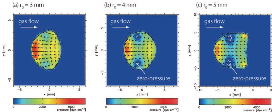
Fig. 16. Internal pressure inside droplet for different droplet radius  $r_0$ : (a) 3 mm, (b) 4 mm, and (c) 5 mm. The pressure at a region surrounded by a white line decreases to almost zero by the eddy. We use  $\mu_d = 1.3$  poise and  $p_{fm} = 4000 \text{ dyn cm}^{-2}$ .
