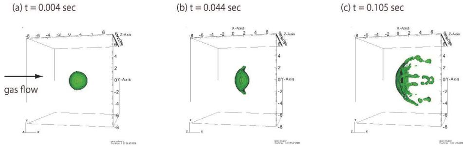
Fig. 15. Three-dimensional view of the fragmentation of molten droplet. We use  $\mu_d = 1$  poise,  $p_{fm} = 4000 \text{ dyn cm}^{-2}$ , and  $r_0 = 2 \text{ cm}$ . The calculation was performed on a  $100 \times 100 \times 100$  grid.
