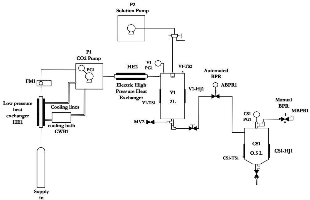
Fig. 4. Schematic diagram of the pilot plant
