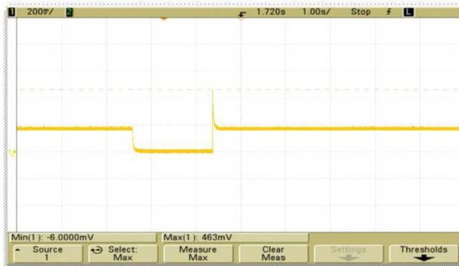
Fig. 14. Voltage waveform at input of boost converter
