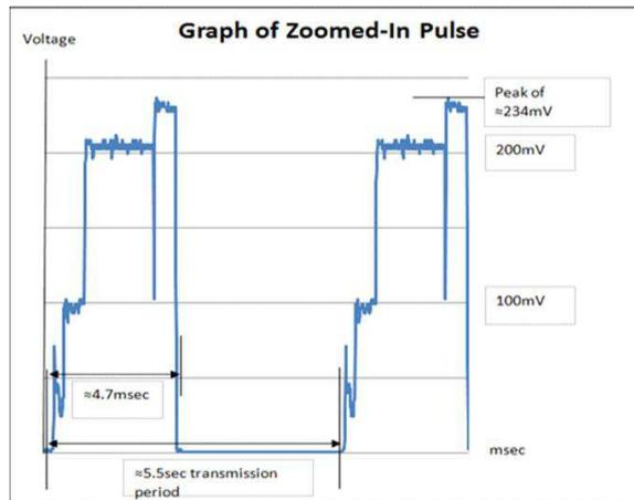
Fig. 10. Zoomed-In pulse current consumption by the TI Target Board with modified configuration of  $\approx 5$  second transmission period. Graph captured across a  $10\Omega$  current sensing resistor in series with load
