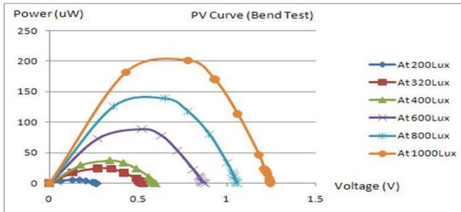
Fig. 21. PV Curves of PV panel at various Lux values when subjected to bending
