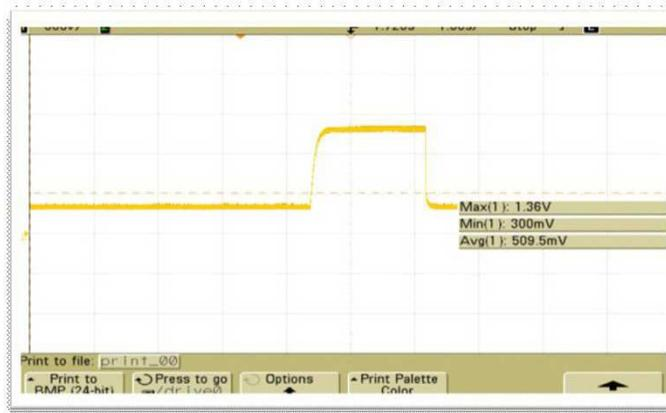
Fig. 13. Voltage across PV panel
