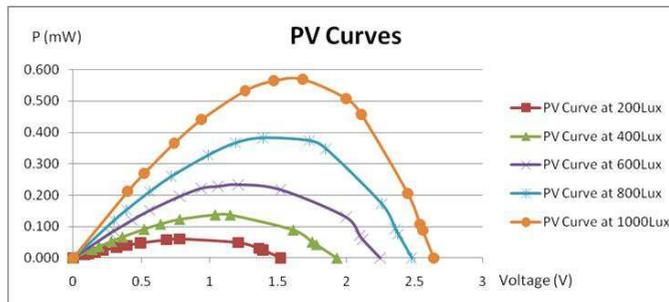
Fig. 6. PV Curves of PV panel at various Lux values
