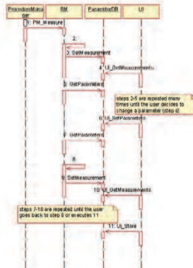
Fig. 6. A parameterization example for the SM capsule. The user changes the SM parameters and the SM reads them through the ParameterDB and applies them in processing. Finally the parameters are saved by the user.
