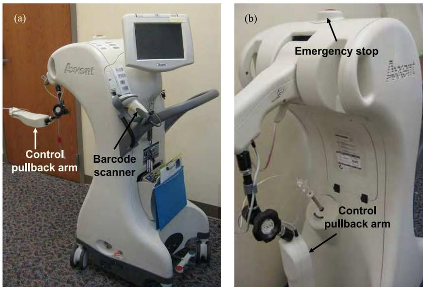
Fig. 1. Axxent Xoift electronic brachytherapy controller with (a) adjustable control pullback arm and barcode scanner; and (b) emergency stop and pullback arm pointing down
