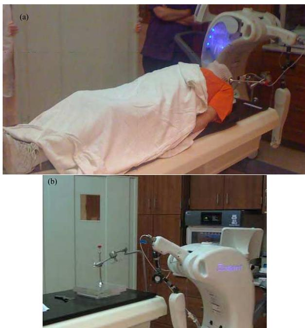
Fig. 10. (a) Patient setup with a thermoplastic facemask for skin treatment on the ear; (b) Radiation protection with the rolling shield in place.
