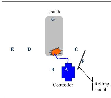
Fig. 11. Diagram of measurement points with clinical setup for ear, scalp and leg cases. Point A is right behind the controller. Point B, G, C, and D are 1 meter from the source superior, inferior, right and left. Point E is 1 meter from the source to the left. Point F is behind the rolling shield.
