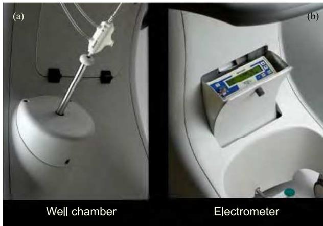
Fig. 2. (a) The well chamber and (b) electrometer are mounted on the controller
