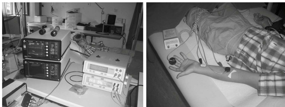
Fig. 2. A typical equipment for assessing skin microcirculation: Laser Doppler flowmeter (LDF, Perimed), the device to register blood pressure in the finger artery (Finapres, Ohmeda), and the transducer for a simultaneous transmission of the digital signals to the computer (left-hand). A typical position of the LDF probes: a standard LD probe (placed on the finger pulp, i.e. representative of glabrous site) and an iontophoretic delivery LD probe (placed on the volar forearm, i.e., representative of nonglabrous area) combined with the device for the application of iontophoresis (right-hand).
