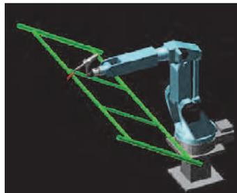
Fig. 16. Computer simulation of scaffold welding process.
