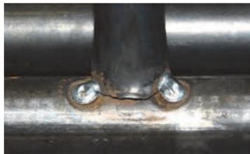
Fig. 22. Arc spot welded joint.
