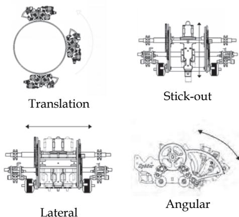
Fig. 31. Degrees of freedom of the robot.
