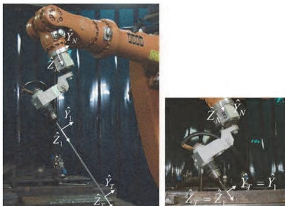
Fig. 8. Complete electrode and melted electrode frames.
