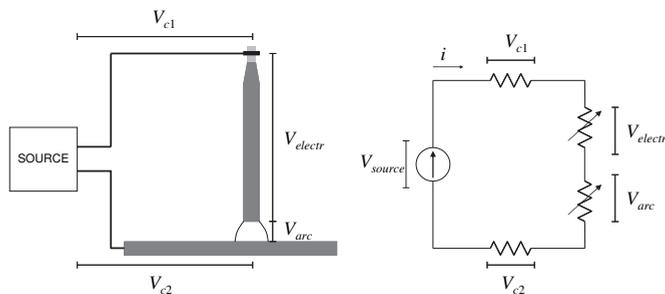
Fig. 7. Electrical circuit of covered electrode welding
