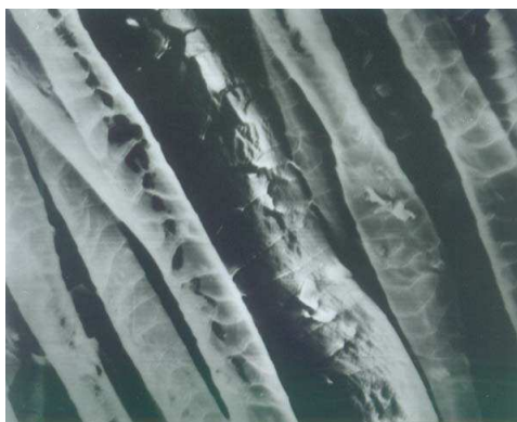
Fig. 1.3. SEM graph of sulphamic acid-treated wool.
