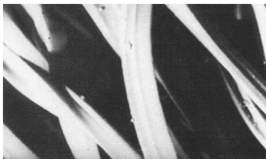
Fig. 2.2. SEM of treated polyester fabric with ethoxide (16) .
