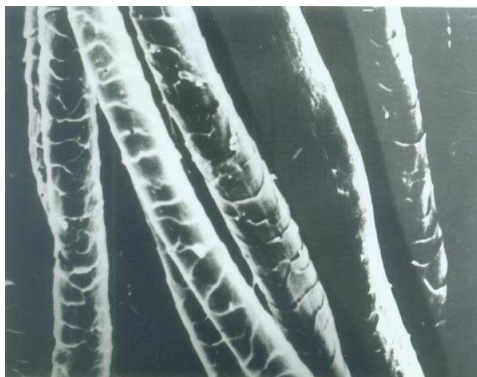
Fig. 1.2. SEM graph of untreated wool.
