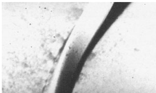
Fig. 2.1. SEM of untreated polyester fabric (16) .
