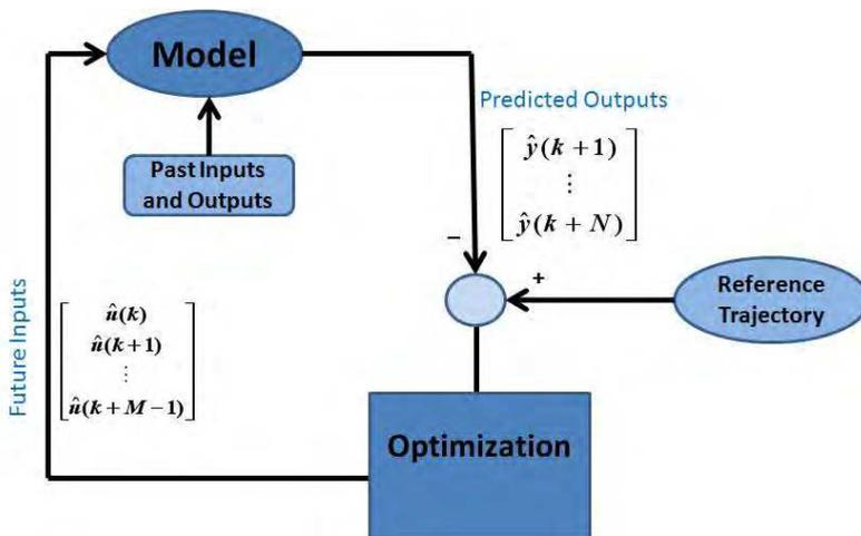
Fig. 1. The stages of the MPC algorithm.
