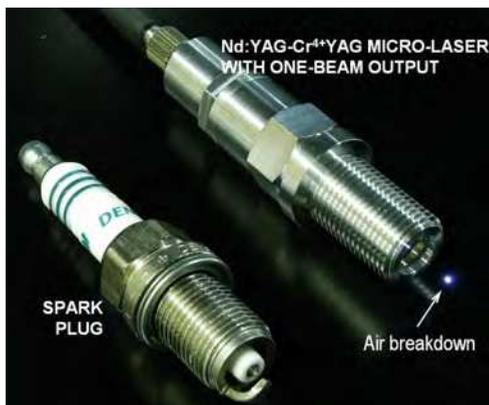
Fig. 9. Nd:YAG-Cr<sup>4+</sup>:YAG laser with one-beam output. Nd:YAG gain medium and Cr<sup>4+</sup>:YAG SA were single crystals; all optical components (including the output mirror) were discrete elements. Air breakdown is shown and size comparison is made with a spark plug.
