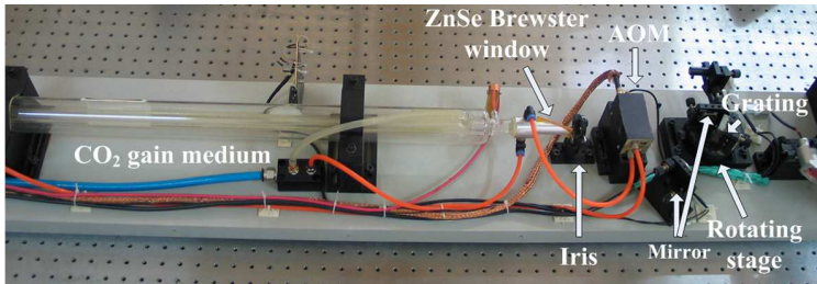
Fig. 16. Tunable acousto-optically Q-switched CO 2 laser
