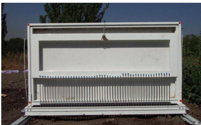
Fig. 1. Pin-meter used to measure soil surface roughness
