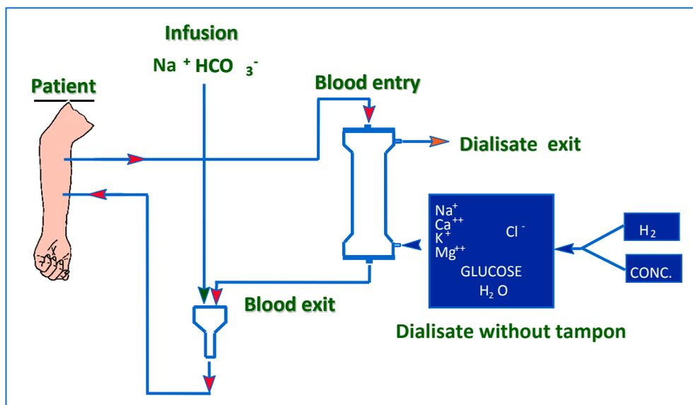
Fig. 1. AFB dialysis circuit.
