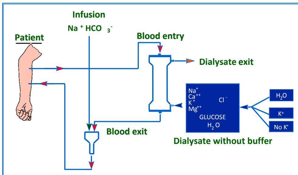
Fig. 2. AFB-K dialysis circuit.
