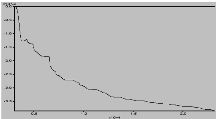
Fig. 4. Displacement convergence of arch crown (Unit:m)
