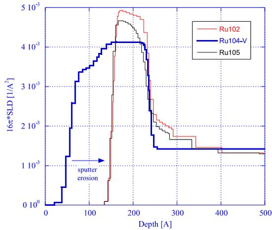
Fig. 15. Electron density depth profiles (ordinate is equal to  $16\pi^2\text{SLD}$ , where  $\text{SLD} = r_e \rho_e$ , and  $r_e$  and  $\rho_e$  are the classical electron radius and electron number density, respectively). The overall film thickness for Ru102 and Ru105 has been reduced by sputtering.
