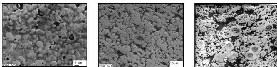
Fig. 3. From left to right, (a) the structure of the W-Cu-Ni-LaB<sub>6</sub> pseudo alloy (x540), (b) the structure of the Cu-44%Mo - 1%LaB<sub>6</sub> pseudo alloy (x2000), and (c) the structure of “irradiated” W-Cu-Ni pseudo alloy produced by class W-Ni powder (x400).
