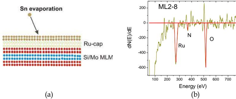
Fig. 9. (a) Schematic of Sn on MLM system. (b) Auger spectra of a thin Ru-cap MLM showing the presence of oxygen on the thin-film Ru cap. This MLM system can reflect up to about 69-72% of EUV light even in the presence of oxygen.
