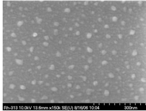
Fig. 14. SEM image of Rh-313 exposed to similar conditions as sample Ru-106. Therefore Sn coverage is equivalent to about a 2-nm thickness of Sn atoms.
