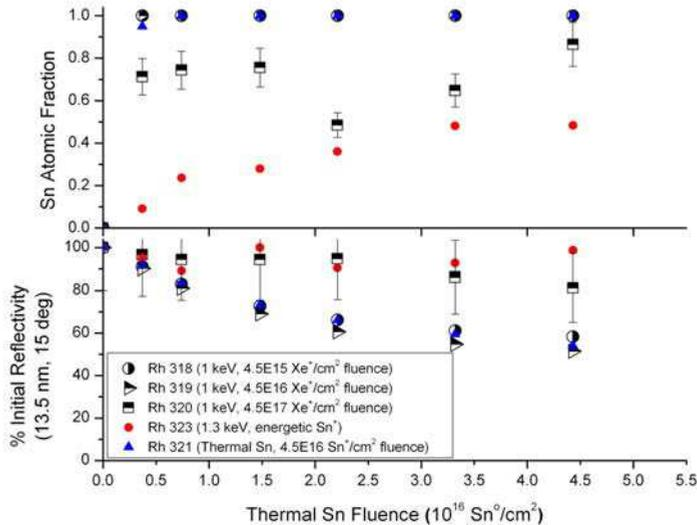
Fig. 20. LEISS data showing the surface Sn fraction versus thermal Sn fluence (top) and 13.5nm EUV reflectivity measurements versus thermal Sn fluence (bottom). Rh 321 had thermal Sn deposition only at a fluence of  $4.5 \times 10^{16} \text{ Sn}^0/\text{cm}^2$ . The fluence of Rh 323 shown, for both cases, is meant for correlation purposes only since there is no thermal Sn fluence on the sample.
