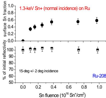
Fig. 19b. Evolution of the surface concentration and the EUV reflectivity of a Ru mirror exposed to a 1.3 keV Sn beam incident at normal incidence (0°).
