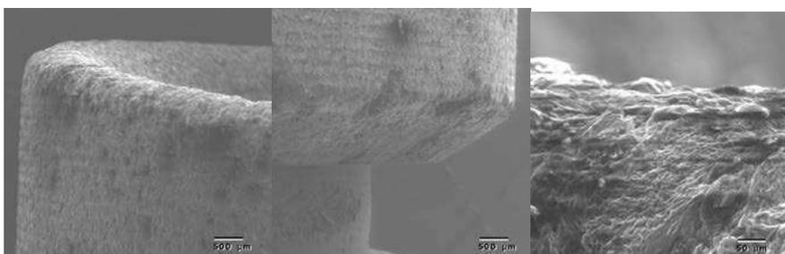
Fig. 2. SEM micrographs of a tungsten electrode exposed to high-intensity plasma during the generation of EUV 13.5-nm light.
