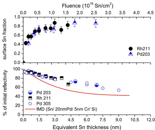
Fig. 16. Evolution of the EUV reflectivity for a Rh mirror as a Sn layer is deposited on the surface compared to deposition on a Pd mirror.
