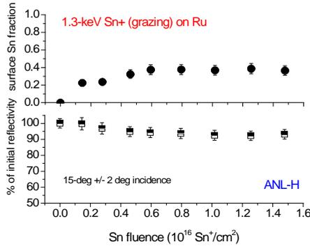
Fig. 19a. Evolution of the surface concentration and the EUV reflectivity of a Ru mirror exposed to a 1.3 keV Sn beam incident at grazing incidence (60°).
