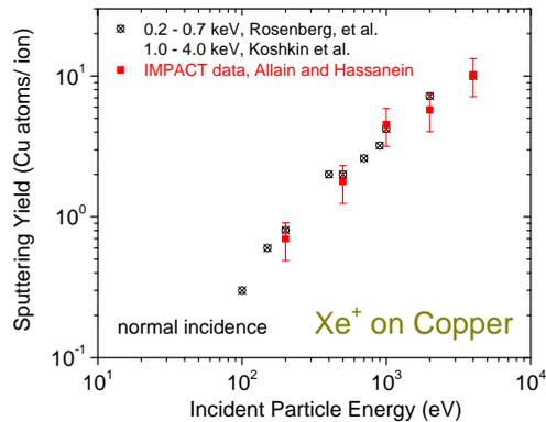
Fig. 5a. Sputtering yield of copper bombarded by singly-charged xenon at normal incidence in the IMPACT (Interaction of Materials with charged Particles And Components Testing) experiment at the Argonne National Laboratory.
