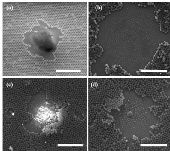
Fig. 11. SEM images for the near-field experiments at fluences above the threshold level: (a) glass substrate ( $F_{\text{peak}} = 7.3$  J/cm<sup>2</sup>), (b) Co thin film ( $F_{\text{peak}} = 0.82$  J/cm<sup>2</sup>), (c) Ag thin film ( $F_{\text{peak}} = 0.18$  J/cm<sup>2</sup>) and (d) Au thin film ( $F_{\text{peak}} = 0.17$  J/cm<sup>2</sup>). Scale bar: 10  $\mu$ m.
