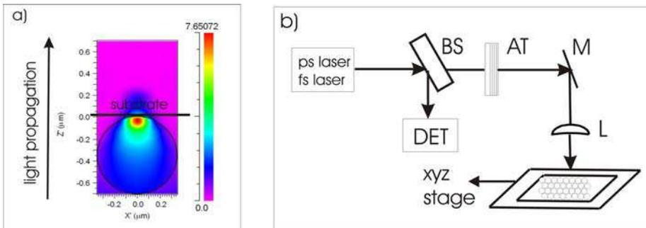
Fig. 10. (a) Field intensity enhancement of a 700 nm colloidal particle sitting on a glass substrate in a free space for  $\lambda = 532$  nm (b) Experimental setup (BS - beam splitter, AT - attenuator, L - convergent lens, DET - pyroelectric detector, M - high reflectivity mirror).
