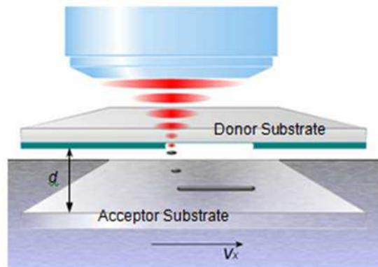
Fig. 14. The schematic of LIFT principle.
