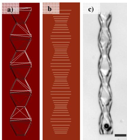
Fig. 3. Description of 3D stereolithography algorithm: a) The design in STL format; b) Computed slices of the 3D design; c) High aspect ratio 3D structure fabricated in Ormoclad. Scale bar: 100  $\mu\text{m}$ . The solid structure is formed by TPP in layer by layer approach.
