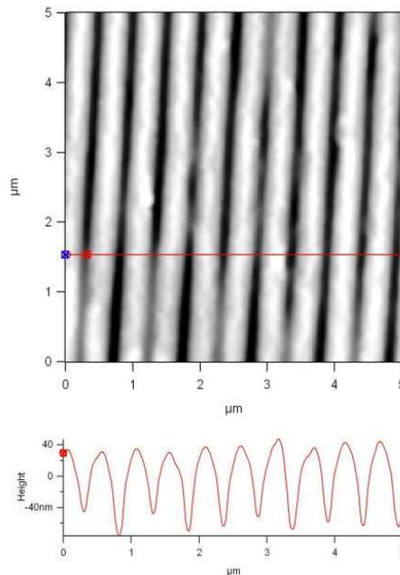
Fig. 3. AFM image of a deformed area on a PDMS stamp. The size of the scanned area is  $5 \mu\text{m} \times 5 \mu\text{m}$
