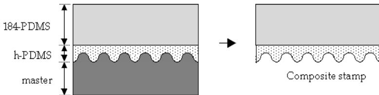
Fig. 8. Configuration of the composite stamp. The h-PDMS is spin-coated on the master template followed by pouring Sylgard 184 PDMS
