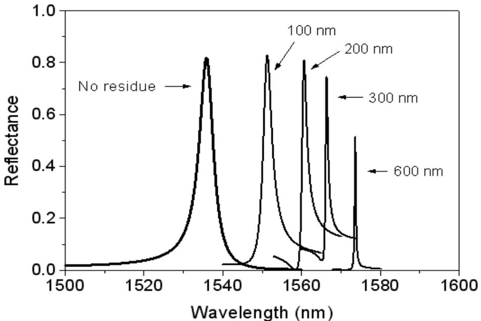
Fig. 12. Calculated spectral response of the fabricated GMR filter with varying thickness of the residual layer ( $d_R$ )
