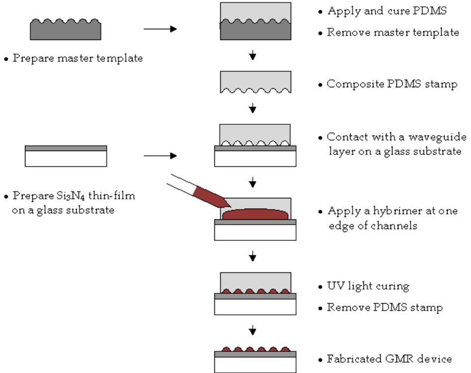
Fig. 7. Schematic fabrication process of a GMR device using the MIMIC method
