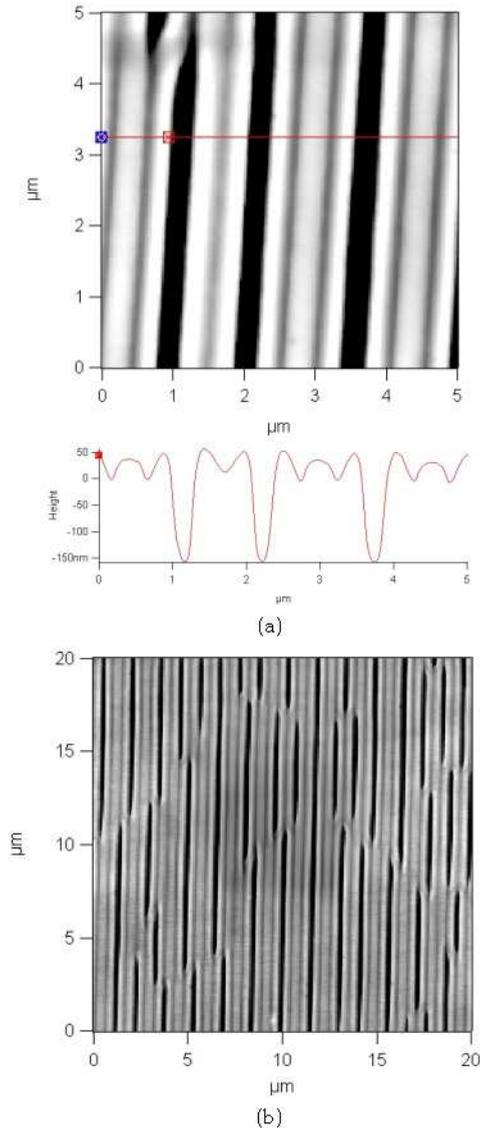
Fig. 4. AFM images of a PDMS stamp having a 520-nm grating period and 220-nm grating depth showing grating-line pairing. The size of the scanned areas are (a)  $5\ \mu\text{m} \times 5\ \mu\text{m}$  and (b)  $20\ \mu\text{m} \times 20\ \mu\text{m}$
