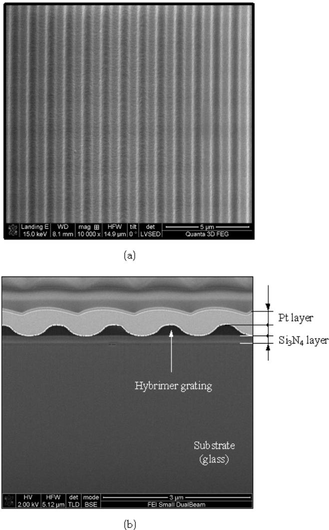
Fig. 13. SEM images of the fabricated GMR device. (a) Top down view, Magnification = 10,000. The size of the image is  $\sim 15 \mu\text{m}$ . (b) Cross-sectional view, Magnification = 25,000. Note that the white part on top is a platinum (Pt) layer for protection during ion-beam sectioning
