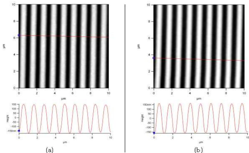
Fig. 9. AFM images of (a) the master template and (b) the composite stamp replica. The size of the scanned area is  $10\ \mu\text{m} \times 10\ \mu\text{m}$
