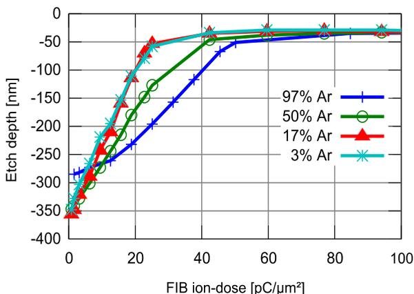
Fig. 11. Impact of the implanted ion dose on the etch depth. The etch gas was composed of Ar and SF<sub>6</sub>.
