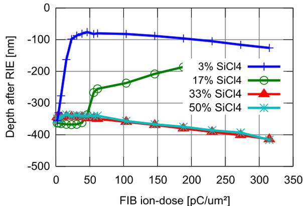
Fig. 17. Impact of the addition of  $\text{SiCl}_4$  to the masking capability of Ga implanted by FIB into Si in a  $\text{SF}_6$ -based RIE process
