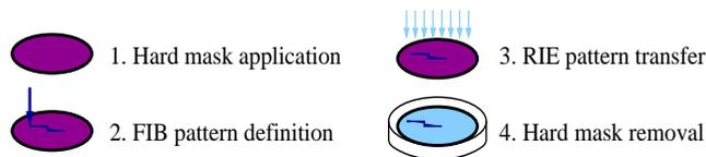
Fig. 14. Process flow for direct hard mask patterning
