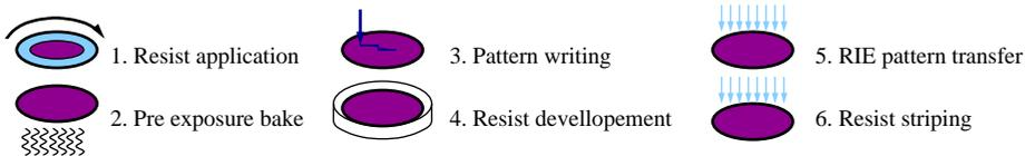
Fig. 8. Typical process flow for resist-based IBL
