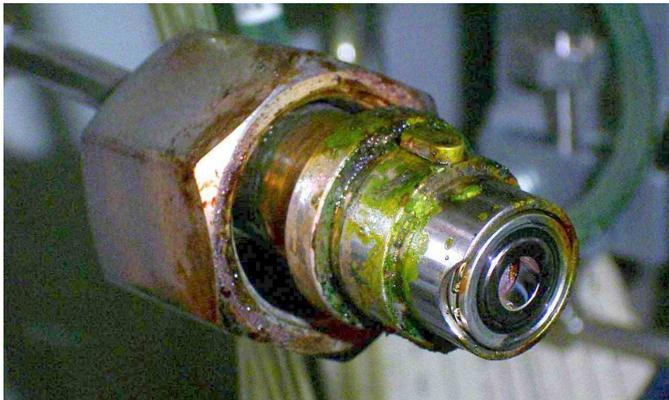
Fig. 6. Green hypochlorous and hydrochloric acids from chlorine corrosion.
