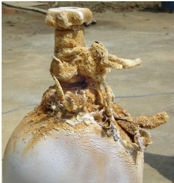
Fig. 2. Typical silane combustion powder.
