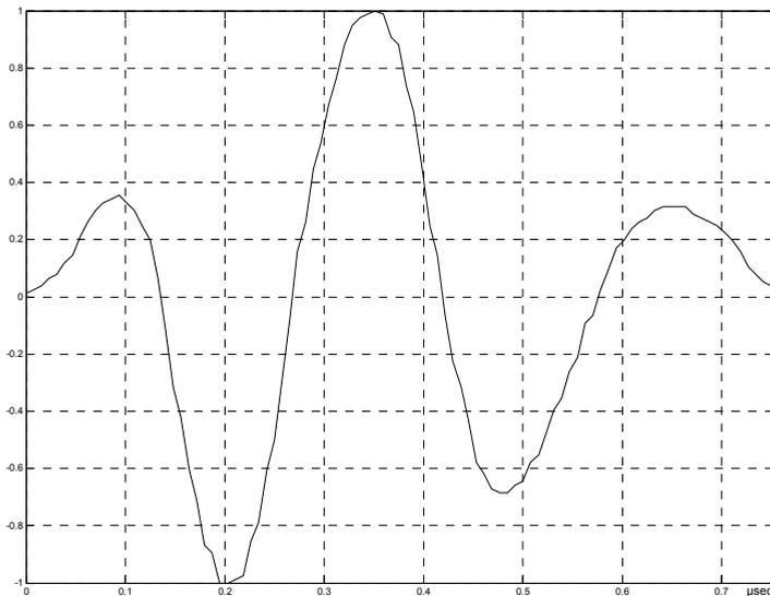
Fig. 5. Ultrasonic echo utilised in type-I experiments.
