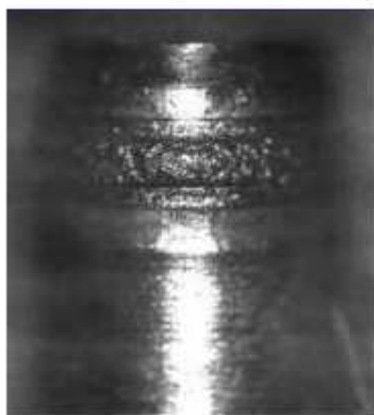
Fig. 8. Optical micrograph (50 times magnified) of a welded capsule.
