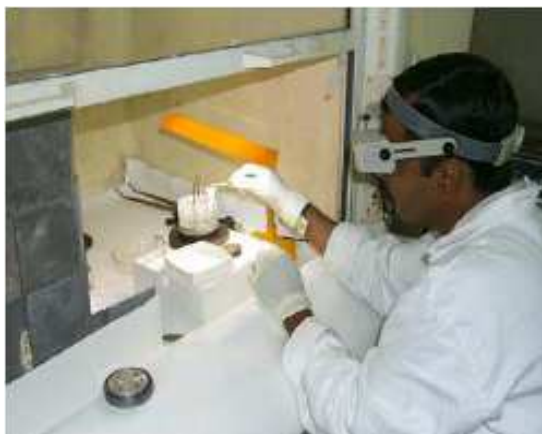
Fig. 5. Loading of ^{125}\text{I} source core inside the capsules
